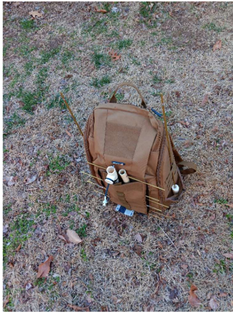
Figure 12 - BACK PACT FOR TRANSPORTING HAM RADIO EQUIPMENT FOR HF THROUGH 432 MHz, INCLUDING RADIO, FEEDLINE, ANTENNAS FOR ALL BANDS, AND MASTS, WEIGHT ~10 LBS.
