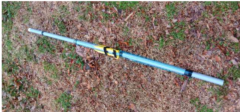
Figure 13 - WALKING STICK/MAST FOR MAN PORTABLE OPERATION TO LOCATIONS AVAILABLE ONLY BY FOOT
