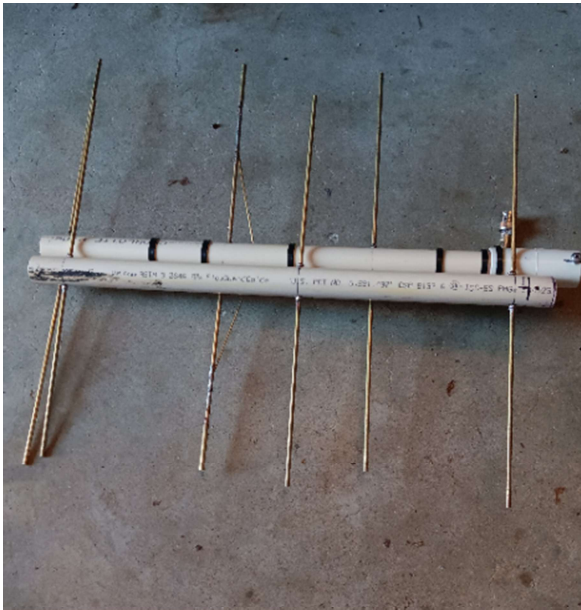
Figure 10 – 432 MHz YAGI DISSASSEMBLED INTO TWO PARTS AND DETAILS OF DELTA MATCH FOR DRIVEN ELEMENT
